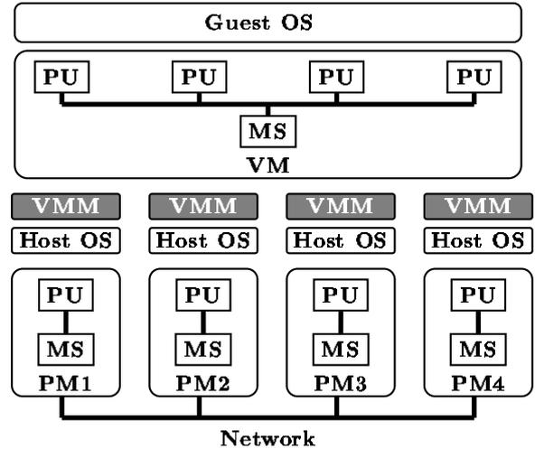
Figure 1: A virtual machine (VM) with four processors built on four single-processor physical machines (PMs). PU and MS denote a processor unit and a main memory (storage) unit respectively.
